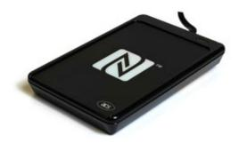
The ACR1252U-MF from ACS is a 13.56 MHz USB-C contactless smartcard reader that supports ISO 14443 type A and B cards, MIFARE, FeliCa, and ISO 18092-compliant NFC cards and tags. This reader is equipped with a SAM slot which provides a high-level of security in contactless and NFC transactions.
